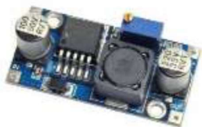
Figure 6. LM2596 dc-dc buck converter
